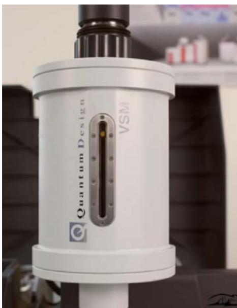
Figure 5. The VSM motor in "load" position.
