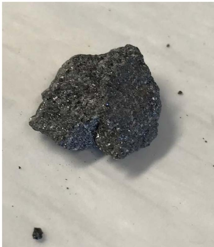
Figure 3. Magnetite with pieces broken off. The small ( $\sim\text{mm}^3$ ) fragments are sufficient for this VSM measurement.
