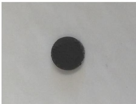
Figure 2. Completed YBCO pellet.
