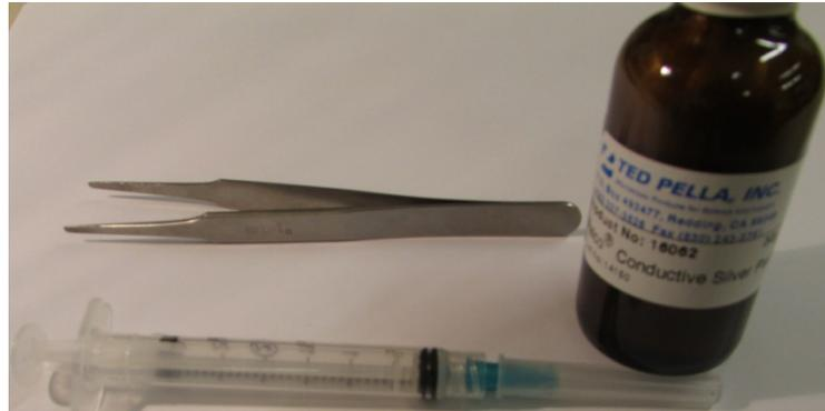
**Figure 5:** Silver paste and syringe for sample contacts
