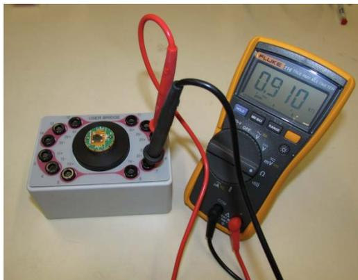
**Figure 8:** Checking sample for continuity
