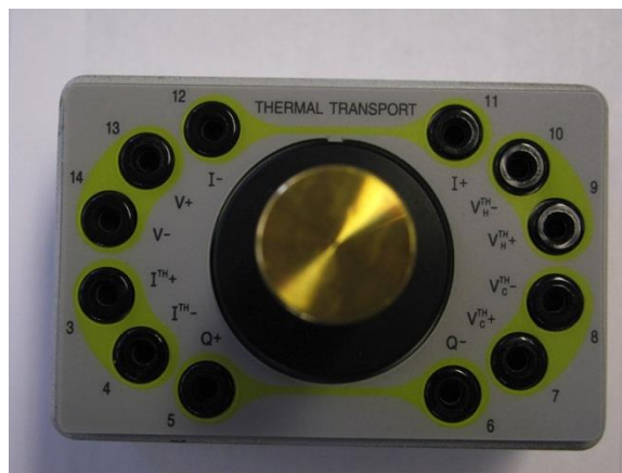
Figure 10: TTO puck on testing box.
