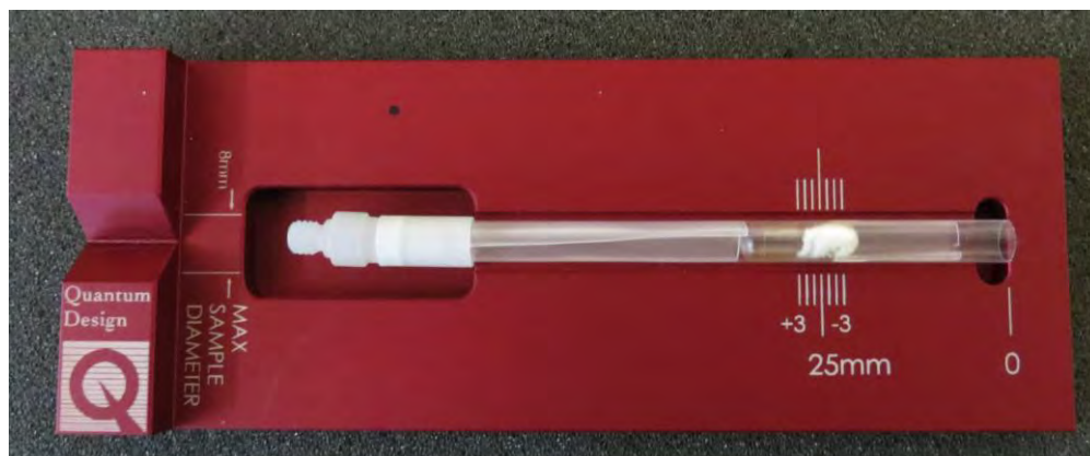
Figure 8: Sample mounting using a #4 gelatin capsule, clear straw, a straw adaptor, and wedging sections of cut straw to hold the sample in place. The sample is wrapped in a small portion of Kimwipe.
