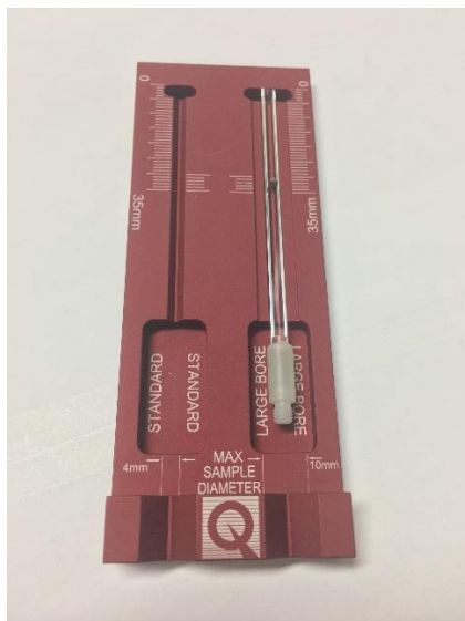
Figure 4. Quartz paddle sample holder with sample in mounting station. The sample is held in place using 7301 varnish.
