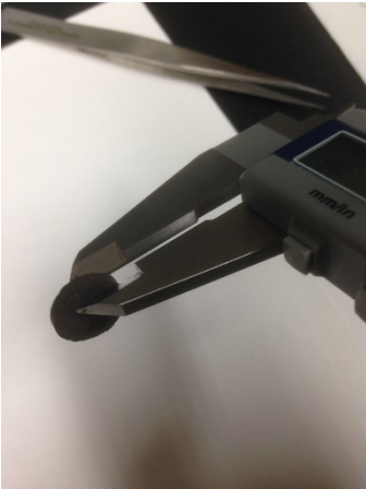
Figure 6. Thickness measurement of pellet in order to determine the cross-sectional area for the resistivity calculation.
